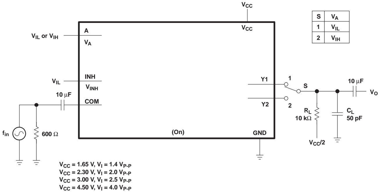
**Figure 10. Sine-Wave Distortion**
